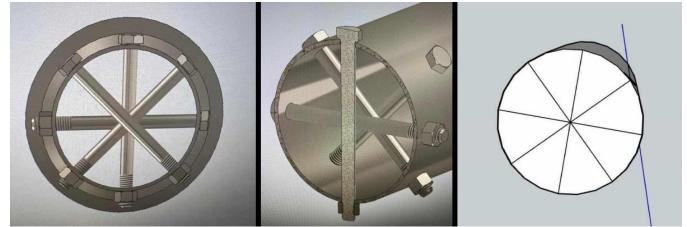
15. All inline turbocharged engines are required to have a cable(s) placed between the first and second cylinders through the exhaust manifold port area. Cable must be a minimum of one (1) 3/8" manufactured pendant line with a rating of at least 3000 lb or more with a tag from the manufacture that indicates rated load capacity with swaged sockets or two (2) 3/8" cables with a minimum of 4 clamps at the splice or crimps with a coupler on each cable. Cable(s) must circle the entire head/block
